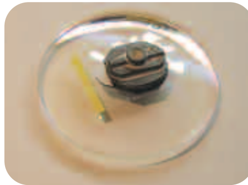
5. Apply transparent blocking pad on the concave side of lens. - Air bubble should be removed between lens and pad
